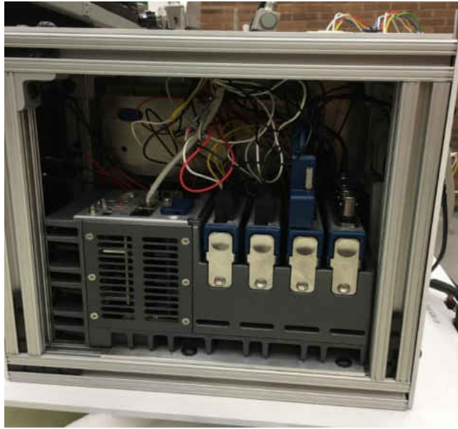
Figure 10: cRIO 9031 DAQ used for balloon flight.
