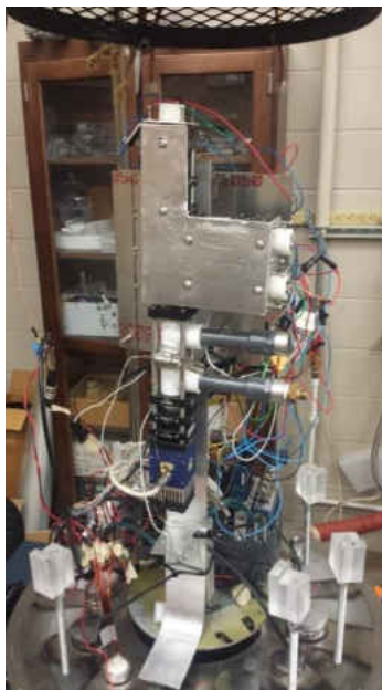
Figure 17: Modified bench top sensor placed inside the test area of a thermal vacuum chamber
