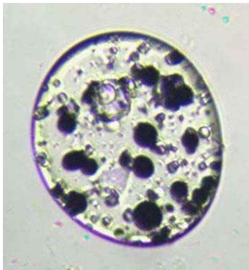
Figure 4 - Micrograph of water-oil-water emulsion droplet containing microscale magnesium particles.
