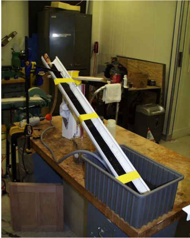
Figure 20 - Emulsion separation process with magnets at regions marked with yellow tape.
