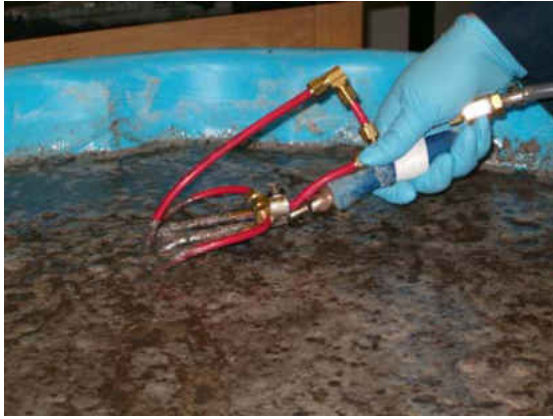
Figure 15 - Action of injected emulsion into sediment.
