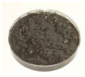
Figure 19 - Sediment mixed with microscale iron emulsion.
