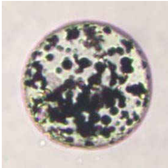
Figure 3 - Micrograph of water-oil-water emulsion droplet containing microscale iron particles.
