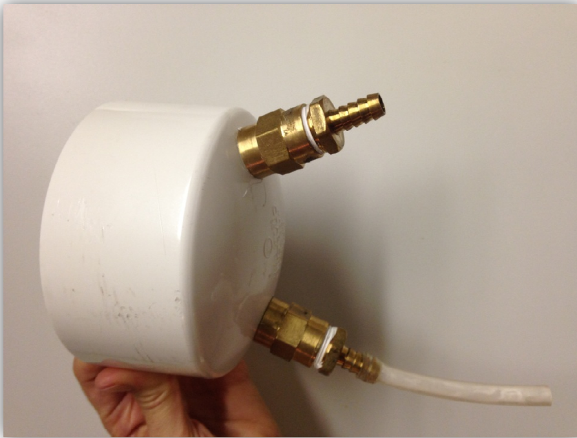
Figure 5: New End Cap with Second Nozzle for Additional Nitrogen, Side View
