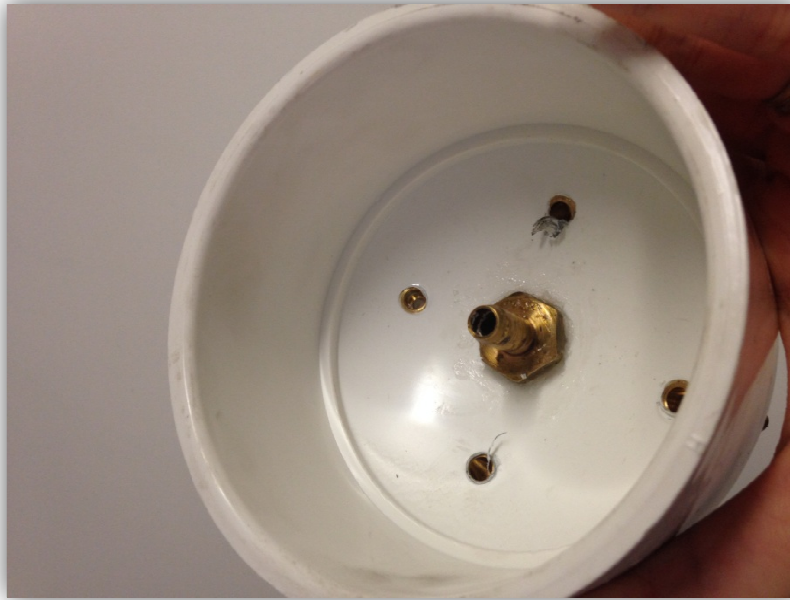
Figure 8: End Cap Reconfigured with Four Perimeter Nozzles for Clean Air Inside View
