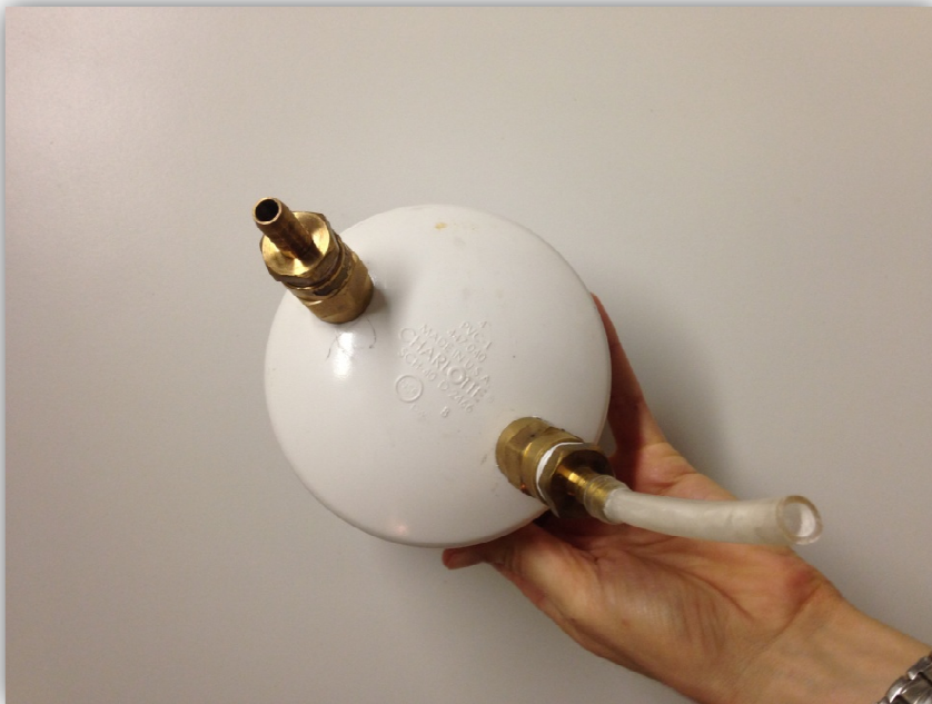
Figure 6: New End Cap with Second Nozzle for Additional Nitrogen - Underside
