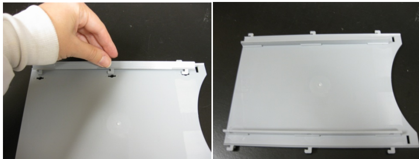
Figure A1 Insertion of the suspension bars. Used for suspending the Radiello sampler.
