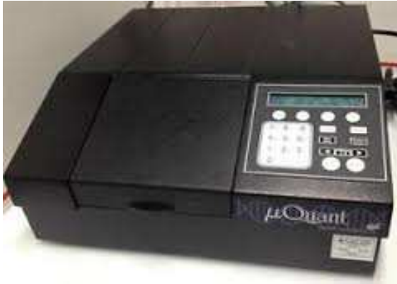
Figure 9. μQuant Spectrophotometer. The spectrophotometer used to read microplates and quantify biochemical medium as the amount of absorbed light that is proportionate to the concentration of the measured solution.
