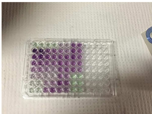
Figure 5. Protein Quantification. A endpoint colorimetric bicinchoninic acid (BCA) assay used to quantify the concentration of protein used for PARP activity analysis.
