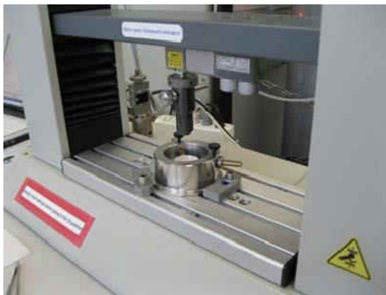
Figure 28. Photograph of the actual instrument used to carry out the ring-on-ring testing [105, 108]
