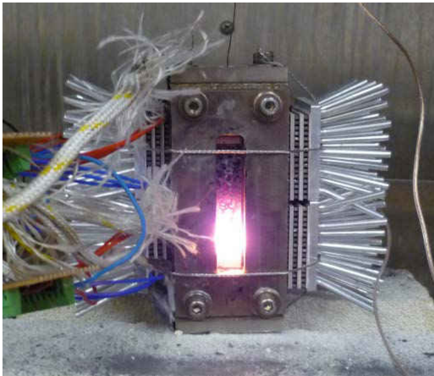
Figure 29: Fully operational assembly of the combustion chamber and TEGs [64].
