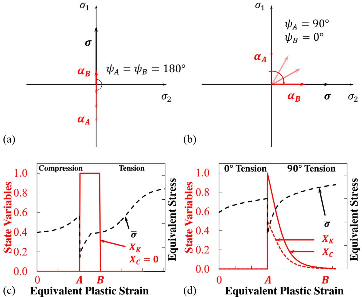
Figure 27 Schematic evolutions of new state variables  $X_K$  and  $X_C$  under (a), (c) reversal compression-tension, and (b), (d) two-step uniaxial tension (cross loading), in the space of (a), (b) stress, and (c), (d) equivalent plastic strain, comparing to their hardening curves.
