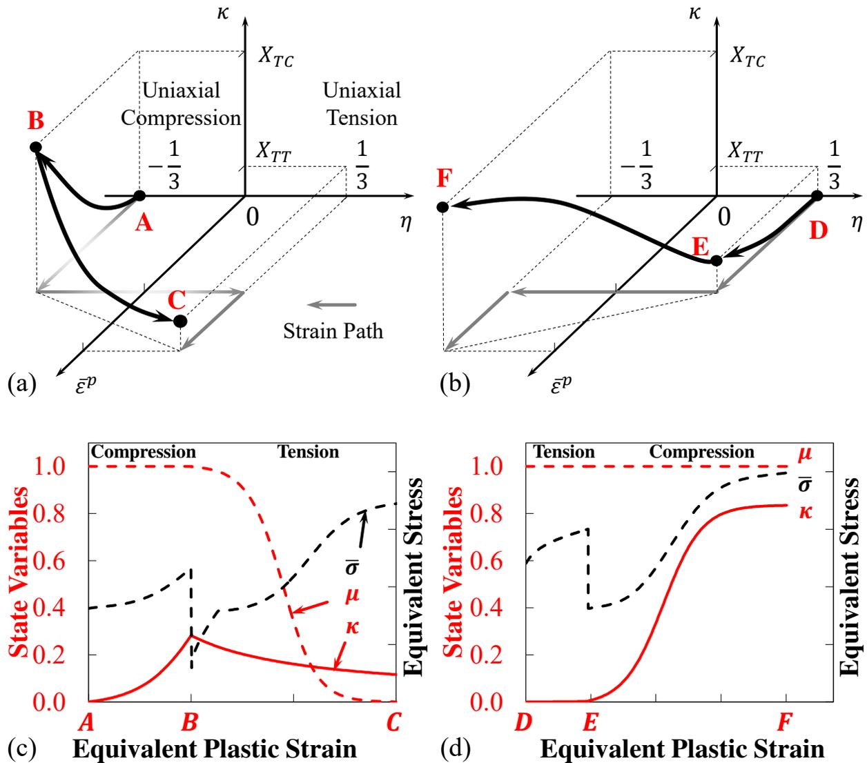
Figure 28 Schematic evolutions of new state variables  $\kappa$  and  $\mu$  under reversal a), c) compression-tension, and b), d) tension-compression, in the space of a), b) equivalent plastic strain with stress triaxiality, and c), d) equivalent plastic strain, comparing to their hardening curves.
