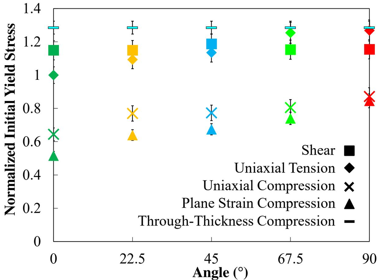
Figure 22 Normalized equivalent stresses versus orientations at initial yield among different loading conditions and orientations. The baseline values are all 220MPa. Error bars of test data are provided.
