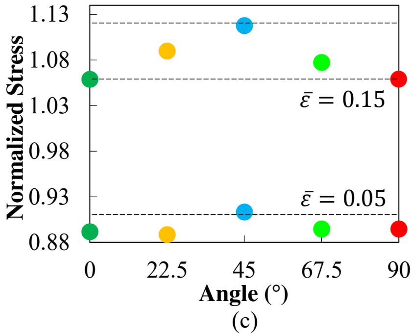
Figure 20 The results for shear tests. (a) Equivalent strain-stress curves, (b) Equivalent plastic strain versus  $\Phi$  angle, the dash line marks pure shear loading condition based on von-Mises plasticity, and (c) Normalized stress at specific equivalent plastic strains. The baseline is 323MPa.
