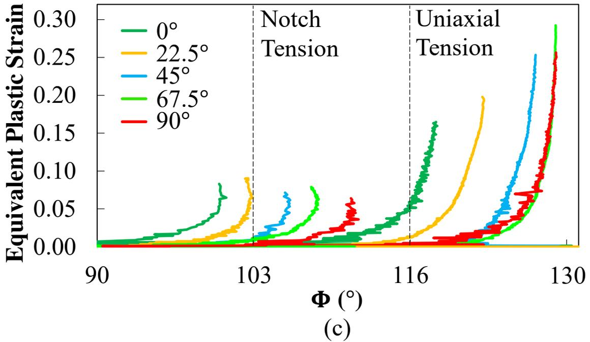
Figure 16 Plastic flow for both uniaxial and notch tension specimens. (a) Lankford ratio versus equivalent plastic strain for uniaxial tension, (b) Lankford ratio versus different orientations for uniaxial tension, extracted at strain level of 0.08, and (c) Equivalent plastic strain versus  $\Phi$  for both uniaxial and notch tension.
