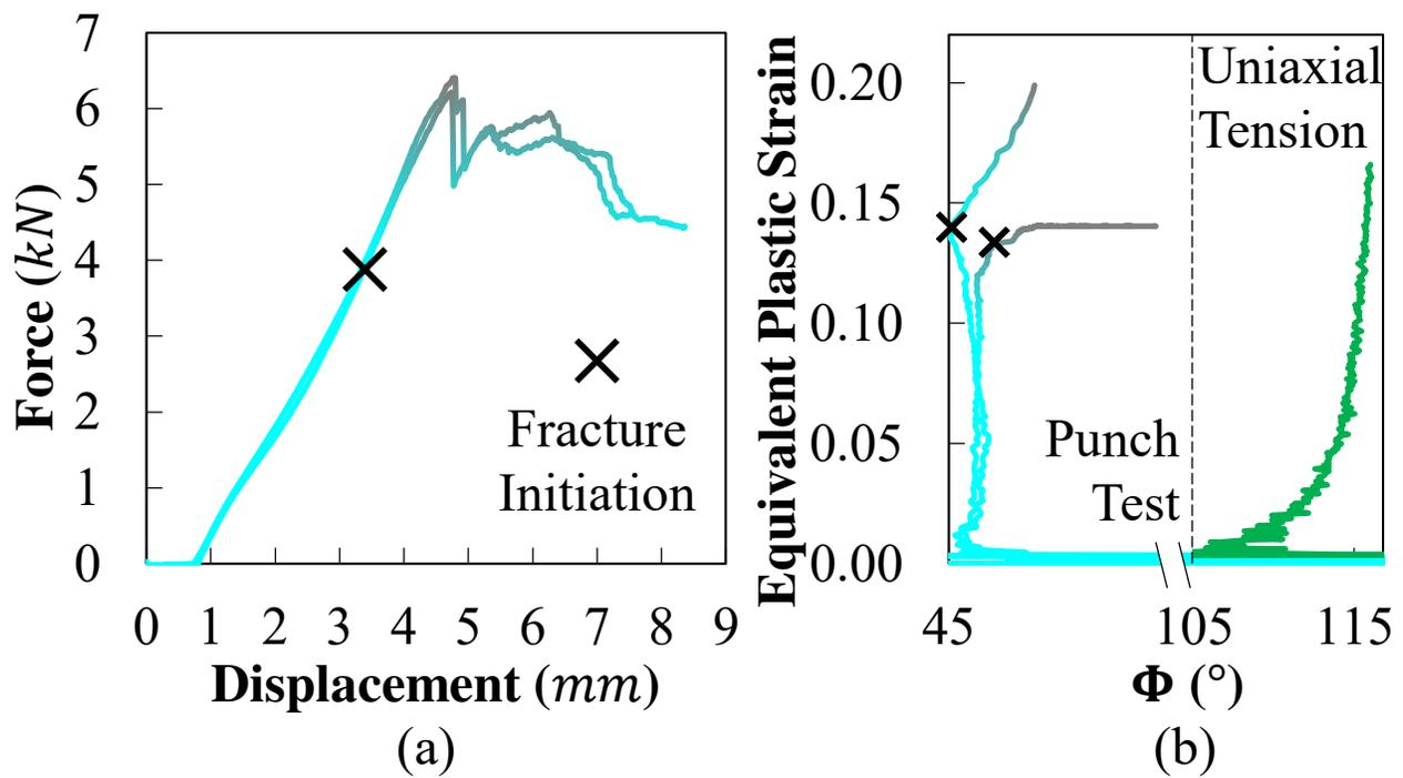
Figure 17 Punch test results, indicating the fracture initiation points. (a) Force-displacement curve, (b) Equivalent plastic strain with  $\Phi$  angle, comparing with the  $0^\circ$  uniaxial tension result. The loading condition change for punch test is distinguished by two colors. (c) The DIC image at the time when fracture initiated.
