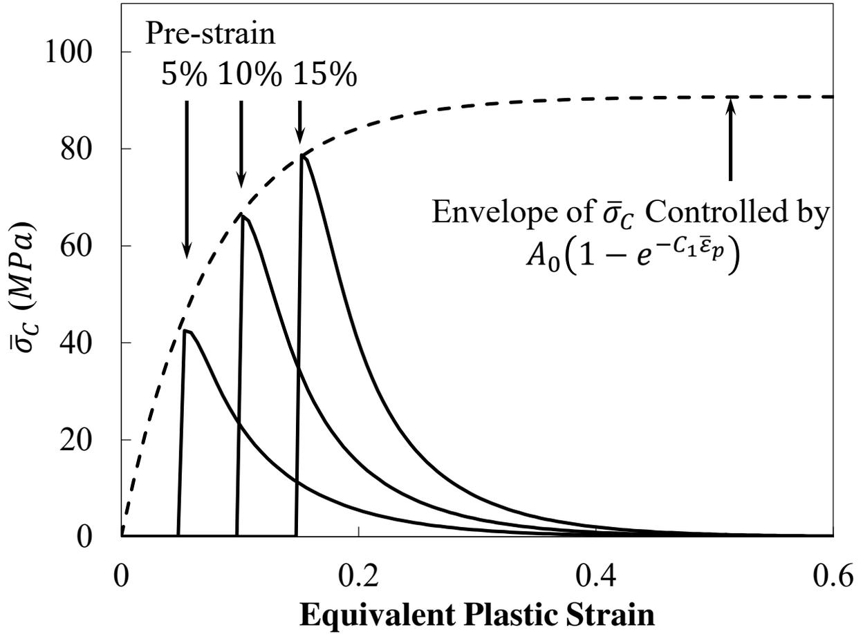
Figure 55 Schematic graph for the adjusted cross-hardening item  $\bar{\sigma}_c$  based on (67). Three different pre-strains, 5%, 10%, and 15% are plotted, with the envelope dash curve of their peak magnitudes.
