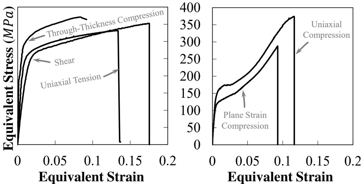
Figure 21 The hardening curves for  $0^\circ$  specimens, comparing with uniaxial tension, shear, through-thickness compression, uniaxial and plane strain compression.
