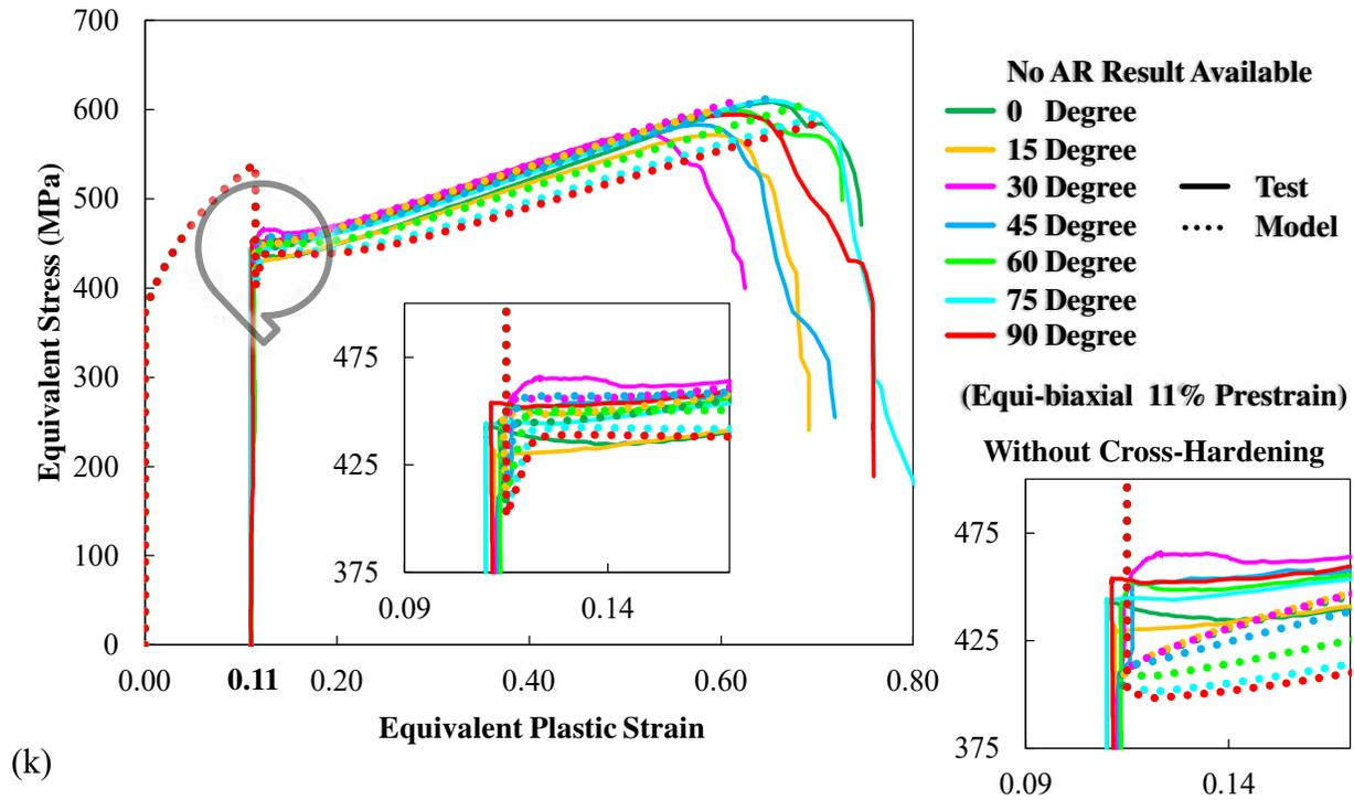
Figure 56 Calibration results for the cross-hardening for the materials of BH240, under the conditions of (a) 5% pre-strain, (b) 10% pre-strain, (c) 15% pre-strain along 0°, (d) 5% pre-strain, (e) 10% pre-strain, (f) 15% pre-strain along 45°, (g) 5% pre-strain, (h) 10% pre-strain, (i) 15% pre-strain along 90° uniaxial tension test, (j) 6% pre-strain, (j) 10% pre-strain of equi-biaxial tension (bulge) test.
