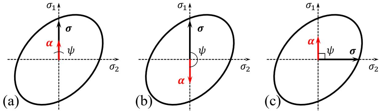
Figure 26 A schematic graph of the angle  $\psi$  in the stress space under (a) monotonic uniaxial tension, (b) reversal uniaxial compression-tension, and (c) two-step uniaxial tension (cross loading).
