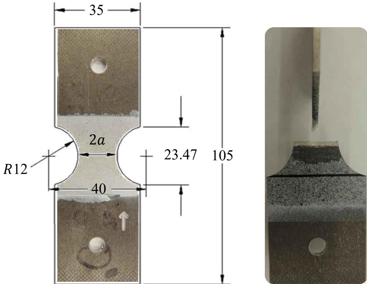
Figure 3 The notch specimen with sizes for biaxial tension. The arrow on the bottom shoulder of specimen on the left figure indicates the rolling direction. All the units are *mm*. The fracture surface is similar with uniaxial tension.
