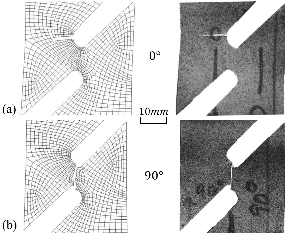
Figure 43 Comparison of the shear fracture modes between experiment and simulation for AZ31B-H24, along (a)  $0^\circ$ , and (b)  $90^\circ$  orientations. The scatters on tested specimens are painted dots for DIC measurement. All pictures share the same scale.
