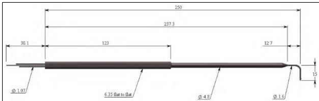
Figure 19: Dimensions of the five-hole probe [2]
