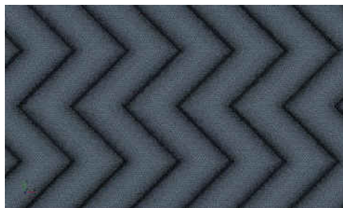
Figure 22 Mesh of the W-2 shaped turbulators
