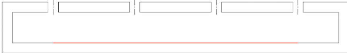
Figure 14 Heated area for the impingement channel
