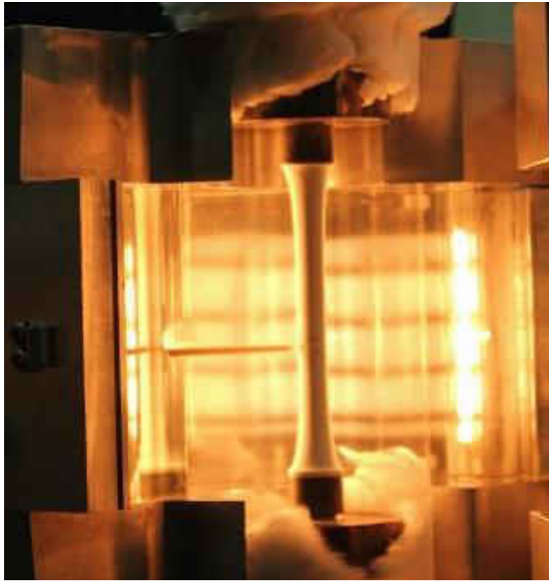
Figure 3.5: Specimen inside radiation heater with visible type S uninsulated thermocouple applied in hoop method for measurement and controller feedback [78].
