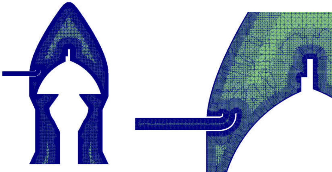
Figure 21: OpenFOAM SnappyHex Mesh Modeling CAD Model of ECS / Spacecraft – 3.5m Configuration (8594480 number of cells)
