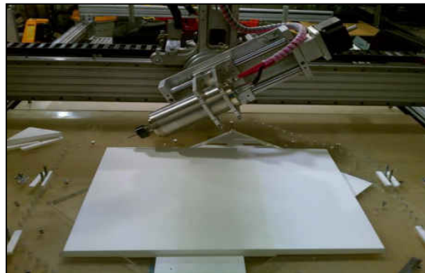
Figure 12: The spindle was rotated to achieve the desired hole inclination angle
