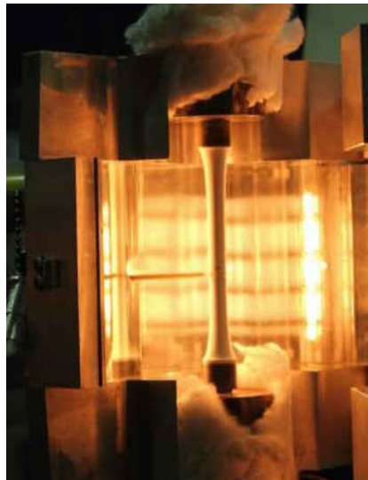
Figure 2.5: Sample heating with surface thermocouple measurement
