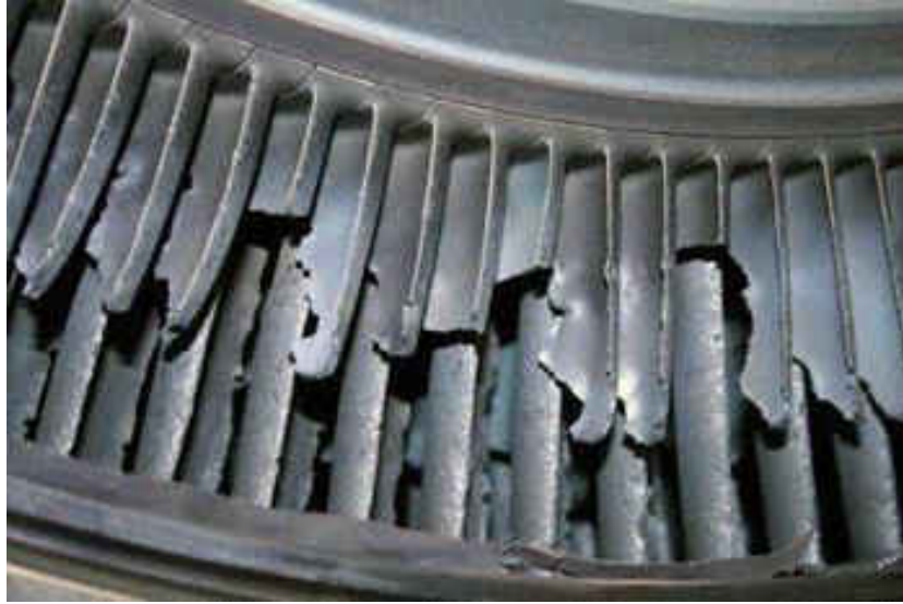
Figure 5. Boeing 737 turbine with blade failure due to thermal degradation of the blades [9]
