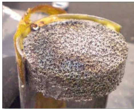
Figure 34) Steel foam as attached to the access hatch of the vaporization chamber.
