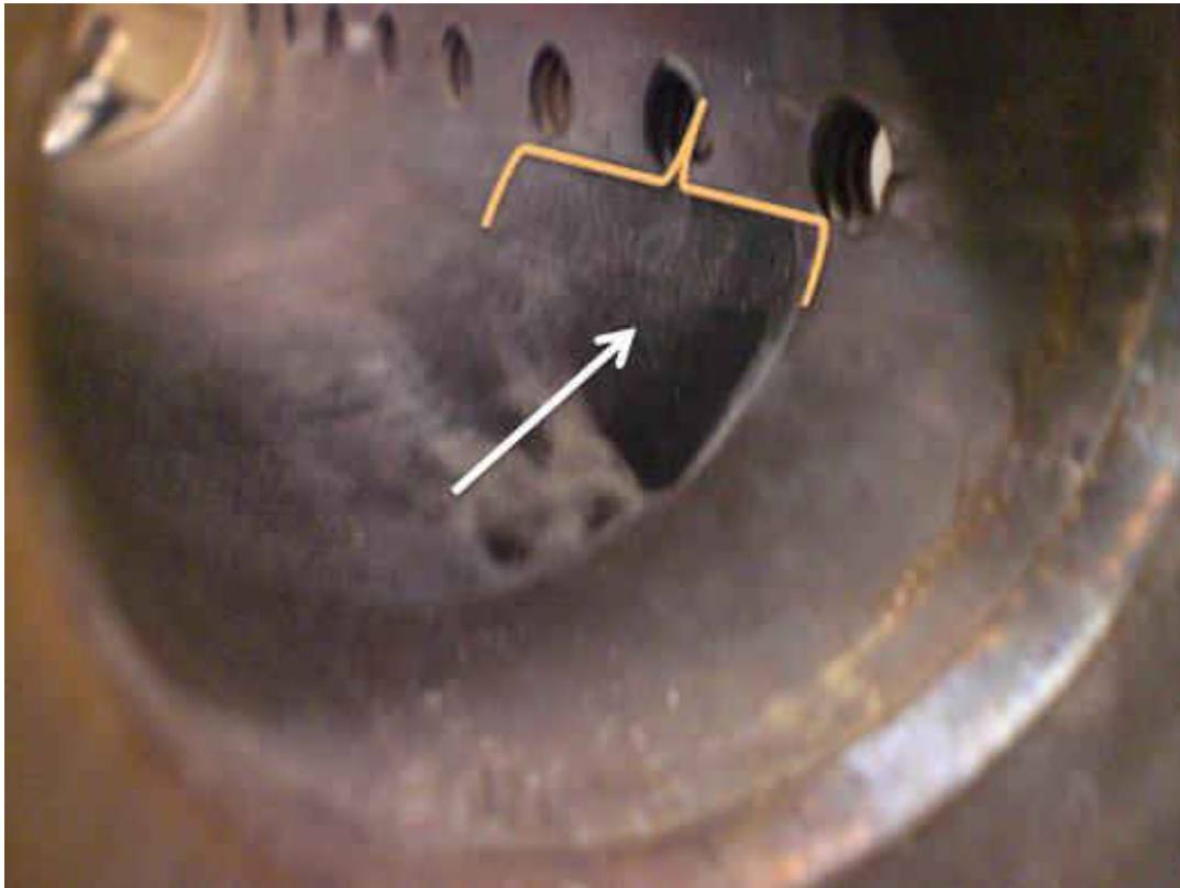
Figure 54) Carbon deposition along the combustion chamber inlet, white arrow pointing to carbon deposition along the wall, with the apparent reaction zone outlined in orange. Spacing between each thermocouple tap center is 2.166 cm.
