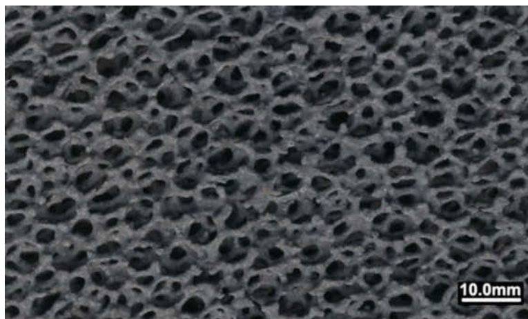
Figure 9) Image of Silicon Carbide Porous Media, ~8.5 pores per linear inch (ppin).
