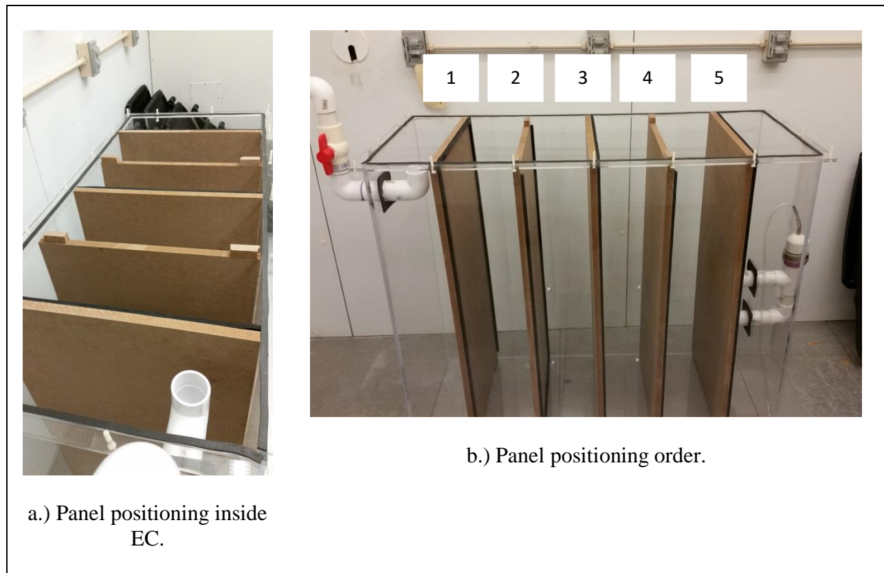
Figure 3. Overview of panel positions inside the EC. a.) Panel positioning inside EC. b.) Panel positioning order.
