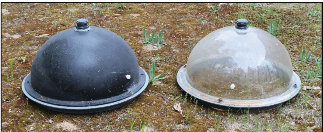
Figure 2. Opaque and transparent benthic chambers. The bottom metal strip was added in 2017.
