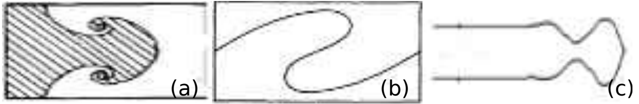
Figure 1.2: (a)Morphology of RTI. Adapted from Kull(1991). (b) Morphology of KHI. Adapted from Rangel and Sirignano(1988). (c) Morphology of RPI. Adapted from Eggers and Villermaux(2008).
