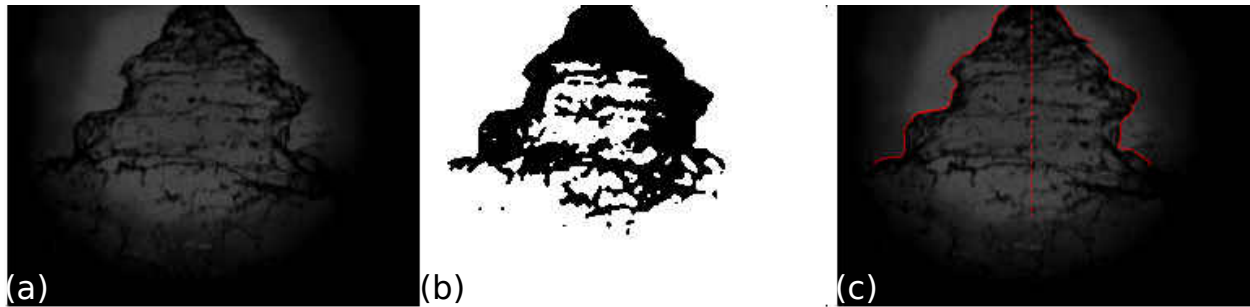
Figure 3.3: Image processing sequence for quantifying the outer interface of the conical film. (a) The original image of a film formed from a nozzle with FN = 8 . (b) Background is subtracted and the image is threshold and converted to binary. The threshold image is such that the film's pixel value is 0, while the rest of the image has a pixel value of 1. (c) The original image with the outer interface traced and the axis located. The solid red line represents radial location of the film for every z location. The dashed red line represents the axis of the film.
