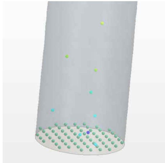
Figure 17 - Particle injection at LVAD inlet.
