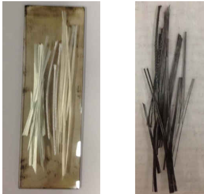
Figure 12 (a) Ceramic fibers before CNTs growth (b) Fuzzy ceramic fibers
