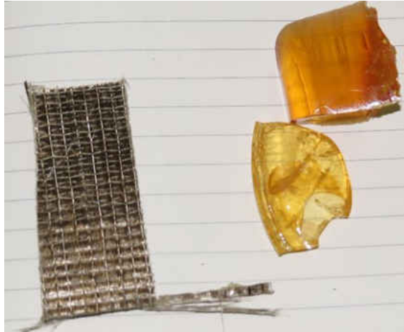
Figure 3: Unpyrolyzed basalt-phenolic laminate
