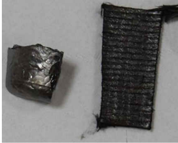
Figure 4: Pyrolyzed basalt-carbon laminate
