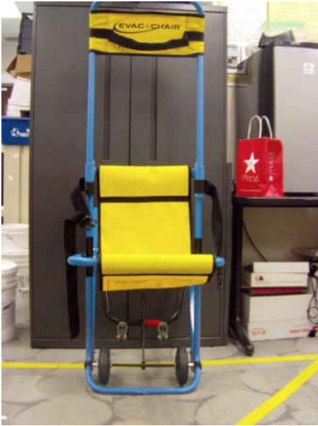
Figure 11: Evac+chair Step 5—Pivot Seat Frame Down
