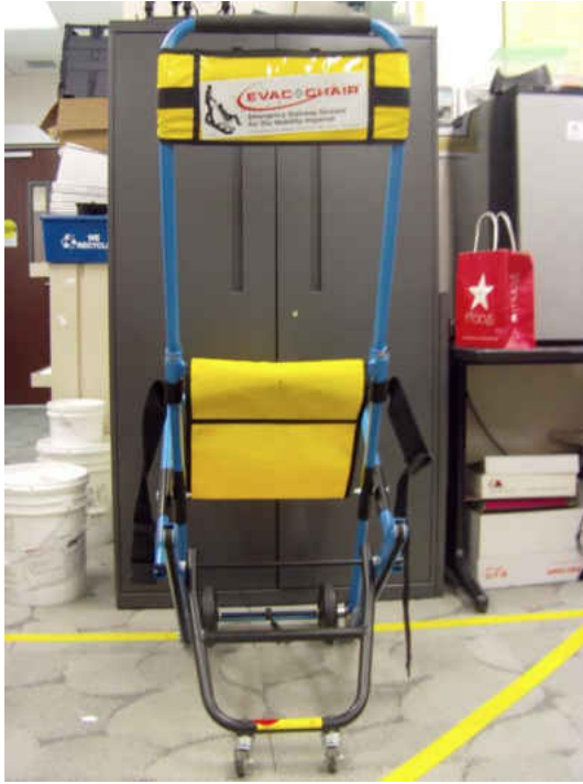
Figure 12: Evac+chair Step 6—Pull Tracks Towards You
