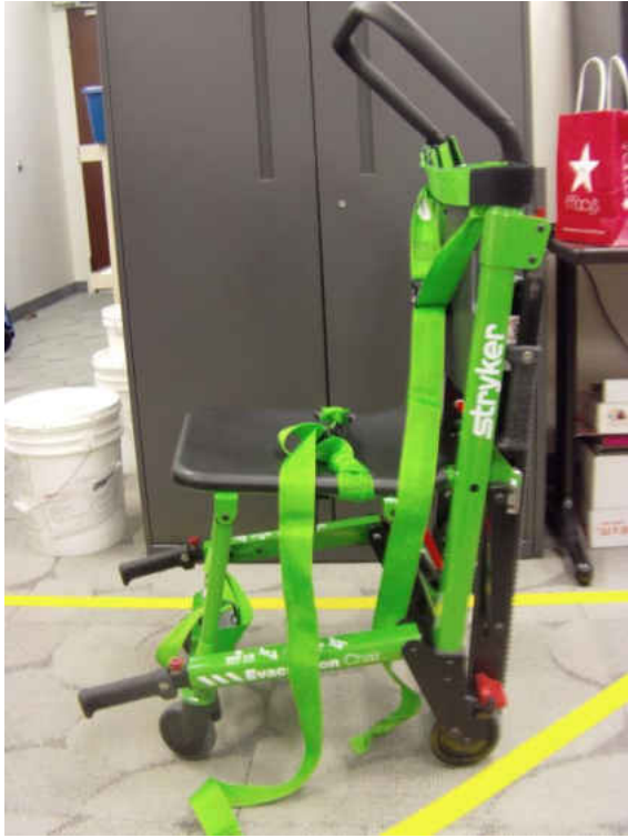
Figure 1: Stryker Step 1—Pull Seat Down
