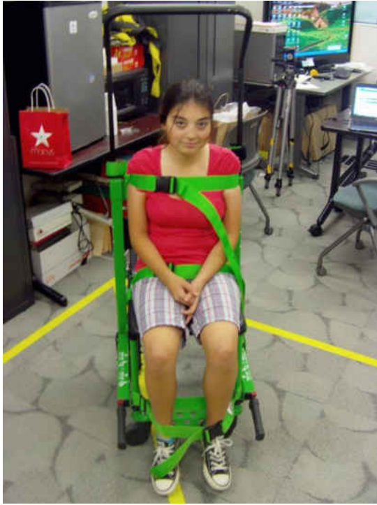
Figure 4: Stryker Step 4—Secure Person Into Chair by Buckling Three Safety Straps
