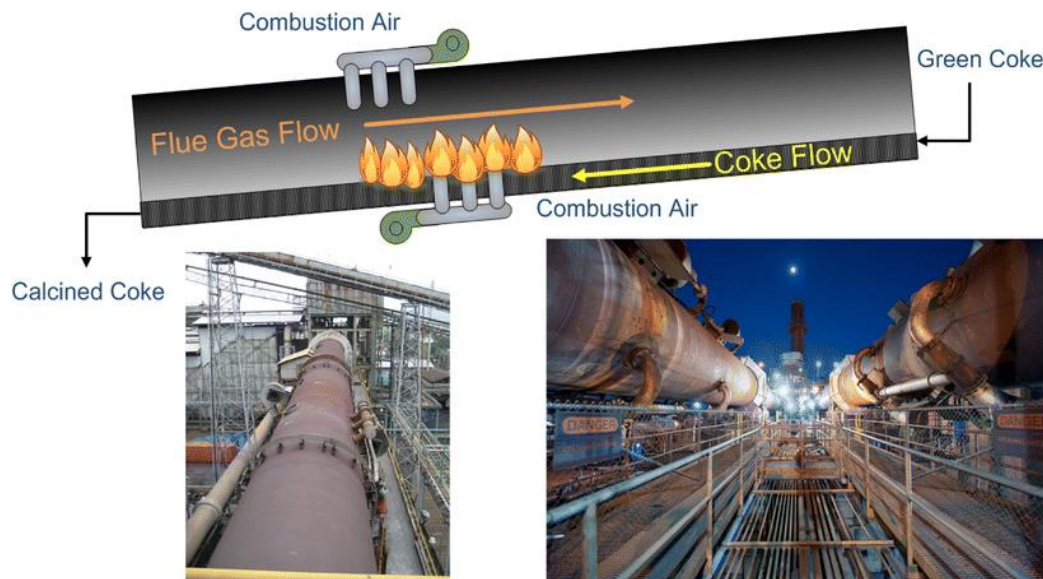
Figure 3 Calcination of Green Coke to Produce Calcined Coke (Edwards et al., 2015) Creative Commons Attribution License
