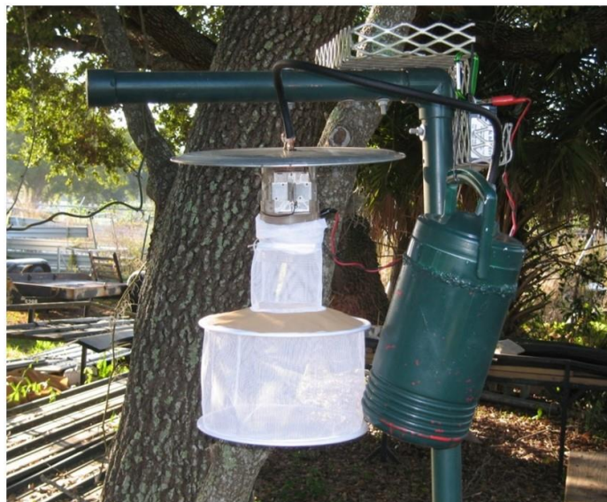
Figure 1: CDC Light Trap Used by Osceola County's Mosquito Control Section Source: Mosquito Control 2014 Update. PowerPoint Presentation. Terry Torrens, Director, Mosquito Control Section, Osceola County.
