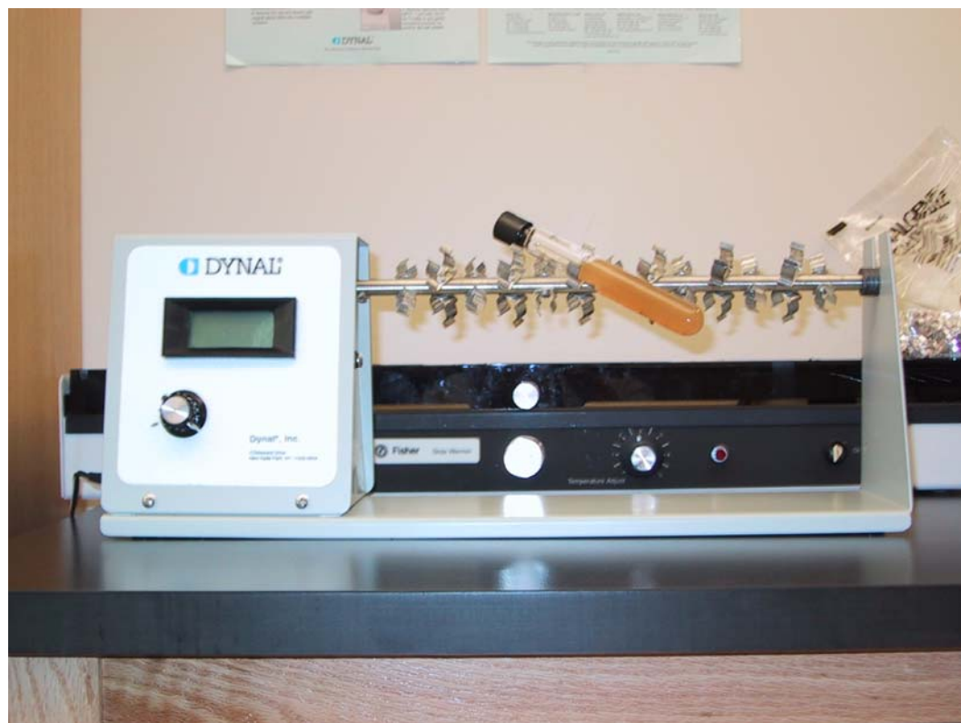
Figure 3 Immunomagnetic separation procedure: Dynal rotation instrument with flat sided tubes mounted
