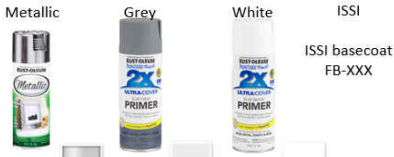
Figure 5.77: Four primers tested to see which combination can best eliminate transmission through the SLA substrate
