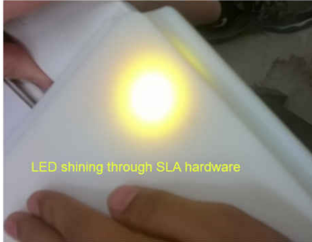
Figure 5.75: LED shining through SLA test hardware
