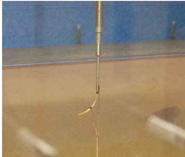
Figure 3.8: Hotwire probe in tunnel at the lowest wall normal position
