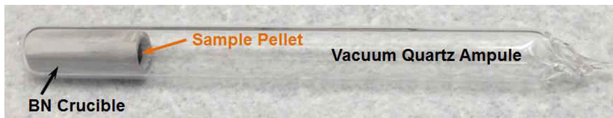
Figure 28: Sealed vacuum quartz ampule with sample pellet loaded in a boron nitride crucible.
