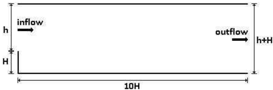
Figure 88: Geometry used in the 2D-DNS on a backward-facing step
