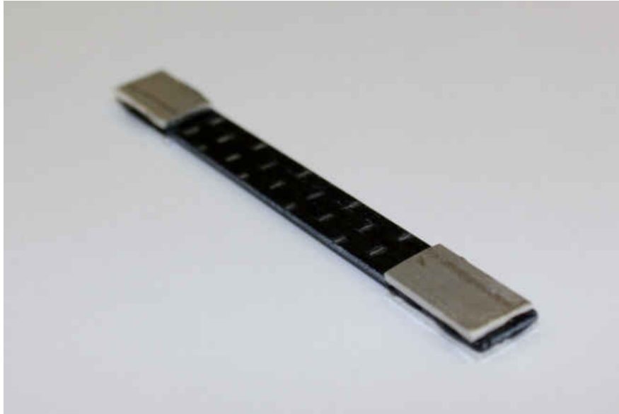
Figure 5.1: Carbon Fiber Specimen with Embedded Alumina Nanoparticles
