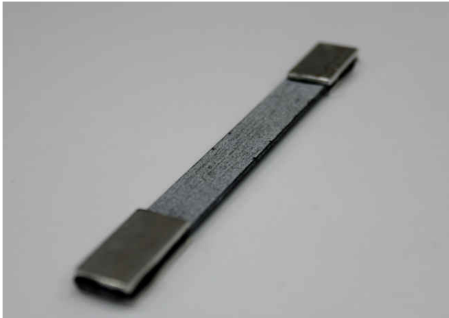
Figure 5.4: DIC Speckles on the Carbon Fiber Alumina Specimen
