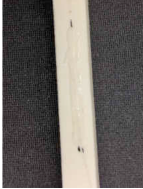
Figure 4.4: FBG Attachment to a Tensile Specimen
