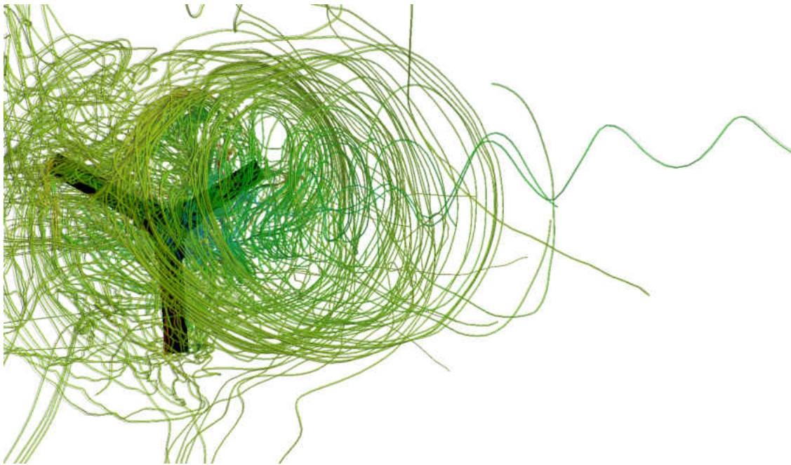
Figure 5.19: Instantaneous streamlines at a free stream velocity of 10\text{m/s} and at an angle of 40^\circ
