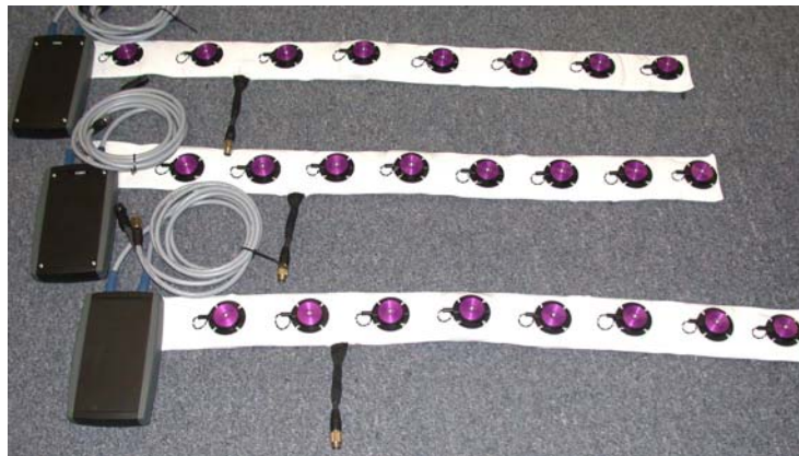
Figure 1. Three tactile displays belt assemblies are shown above along with their three controller boxes.
