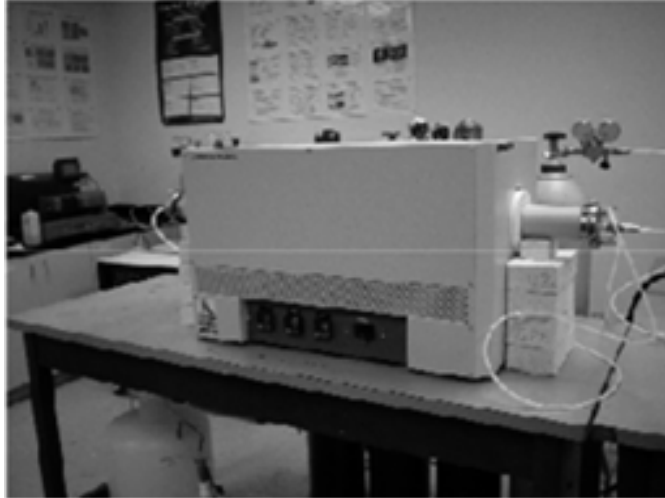
Figure 10. Lindberg/Blue™ three-zone tube furnace used for the heat treatment of alloys and diffusion couples.
