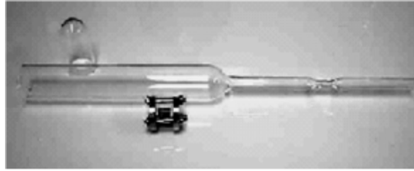
Figure 7. Quartz capsule for heat treatment of diffusion couples, and a diffusion couple jig assembly holding a diffusion couple before diffusion anneal.
