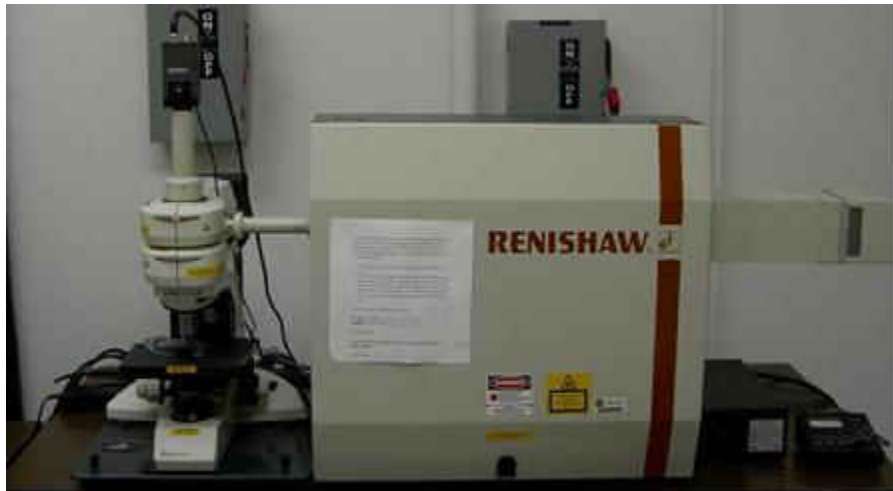
Figure 42. Renishaw TM 1000B Raman Microscope used for performing PLS measurements in this study.
