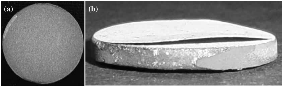
Figure 58. Macro photographs illustrating failure mode of type II APS TBCs with NiCoCrAlY bondcoat with average lifetime of 286 cycles: (a) top surface of bondcoat after YSZ spallation that (b) occurred with initial damage at the edge of the button.
