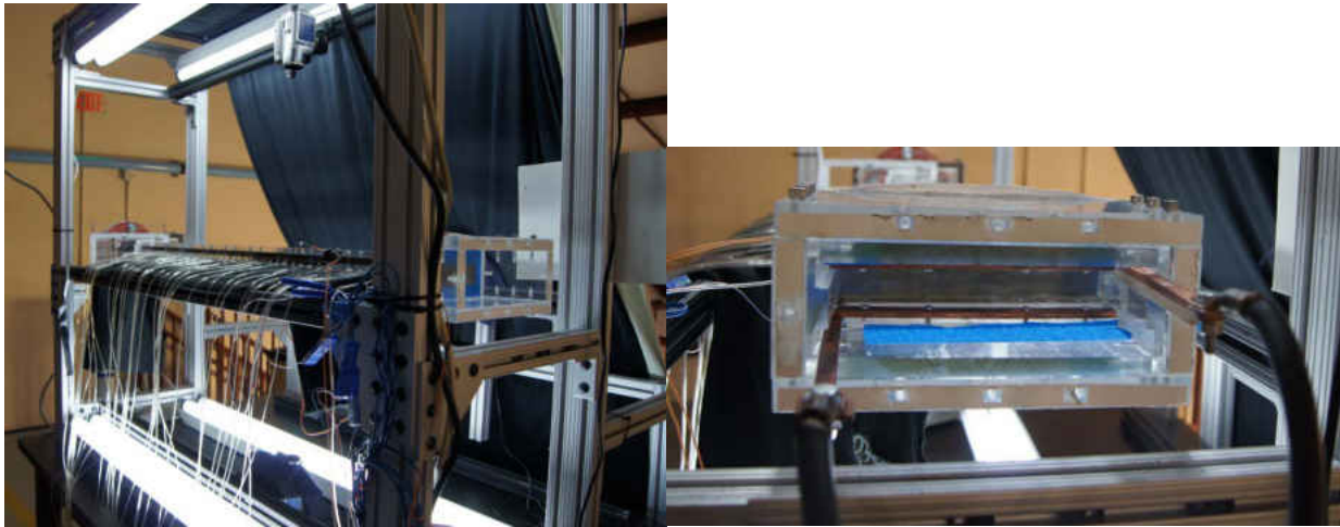
Figure 22: TLC Channel Setup & Inlet Heater Box
