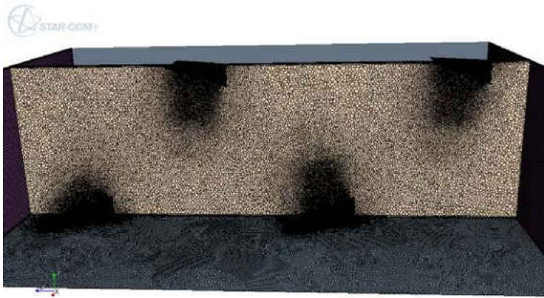
Figure 31: y+ Values on Wedge Surface
