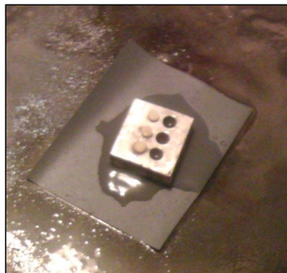
Figure 3.3: Surface finishing using an aluminum jig
