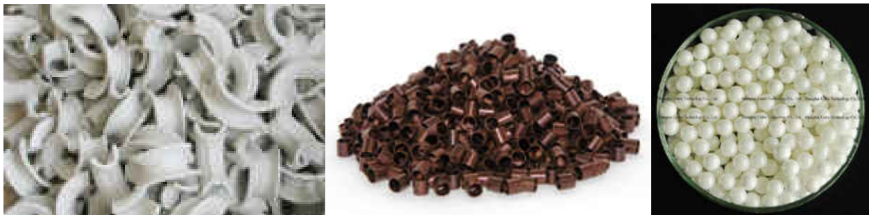
Figure 7. Packed bed geometries: saddles, Raschig rings and spheres [38,39,40]
