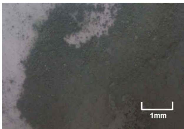
Figure 57 - Anode sample sintered with polyethylene which caused reduction of NiO to Ni during sintering.
