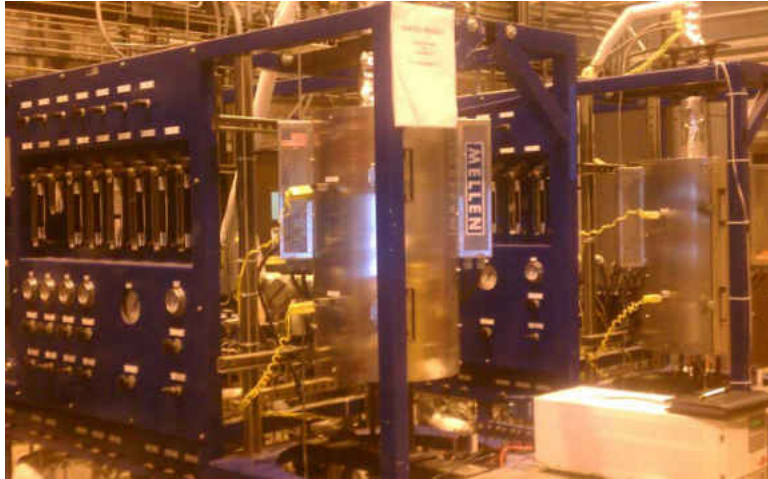
Figure 40 – NETL custom built single cell test stand.
