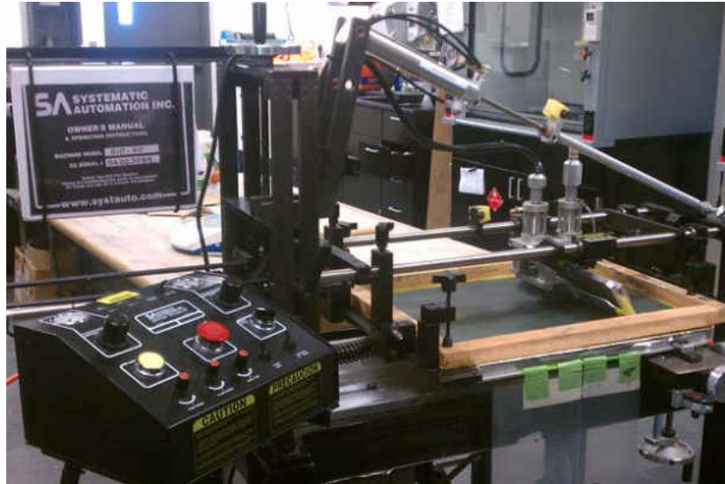
Figure 37 - Screen printing apparatus for application of electrodes to electrolyte.
