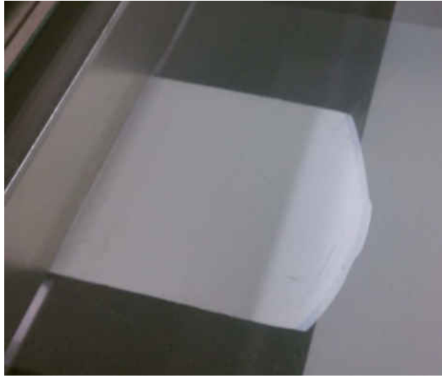
Figure 47 - Green tape being cast.
