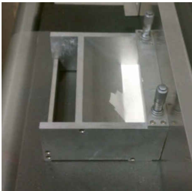
Figure 46 - Slurry in doctor blade.
