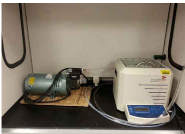
Figure 35 - Spin-coater with vacuum pump set up in ventilation hood and connected to building air supply.
