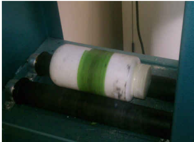
Figure 29 - Ball milling of slurry to ensure proper mixture of all components.
