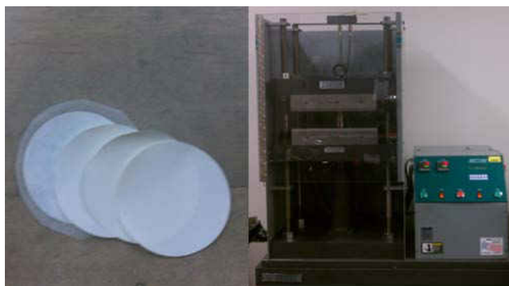
Figure 34 - Laminating and pressing of green tape discs.
