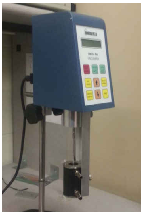
Figure 38 - Brookfield DV-II+ Pro viscometer.
