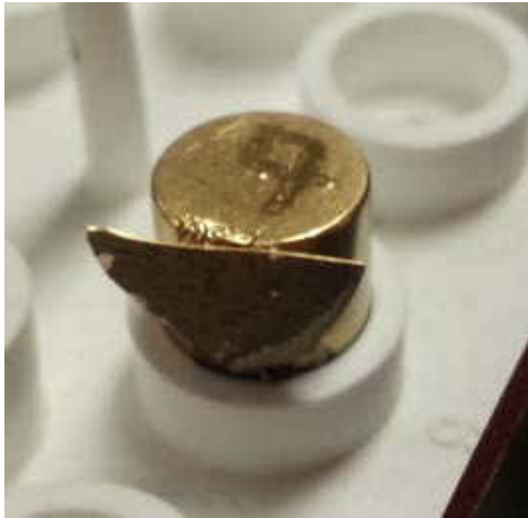
Figure 42 - SOFC fragment held on metal sample holder with conductive carbon tape and sputter coated in gold to make SEM possible.
