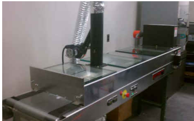
Figure 30 – ProCast tape casting machine for producing electrolyte green tapes.
