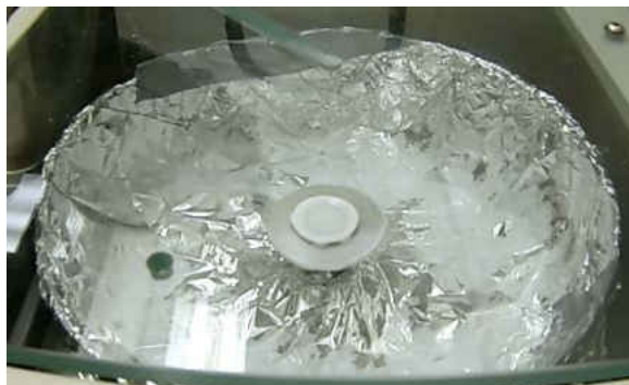
Figure 51 - Spin coating electrolytes with GDC.
