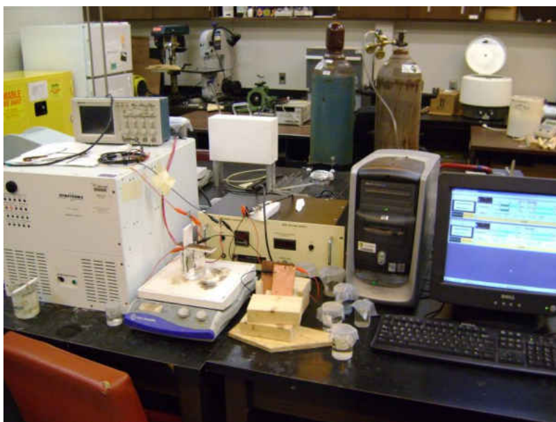
Figure 26: Experimental electrochemical deposition setup
