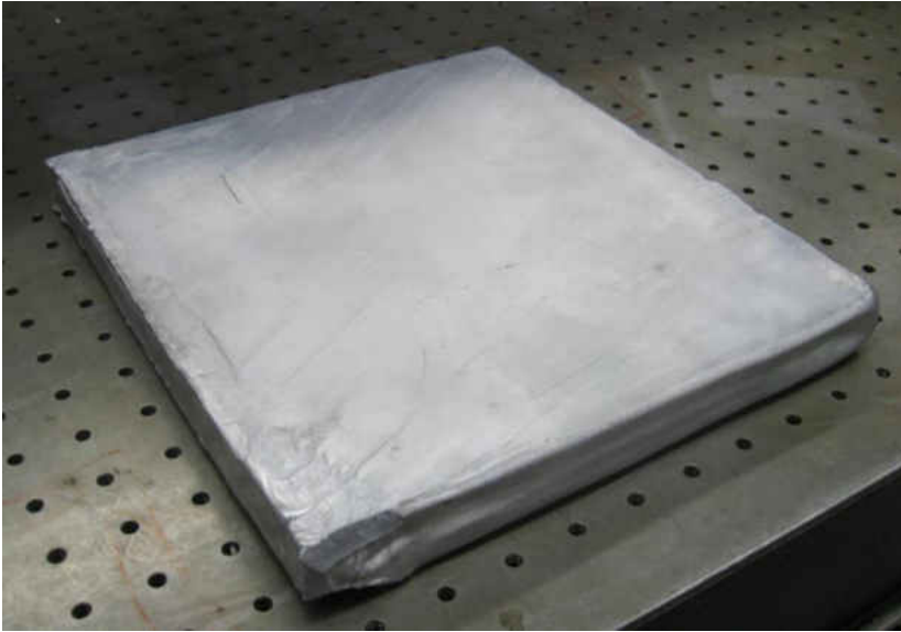
Figure 1.1: 12 in x 12 in cast slab of A359-SiC p -30%
