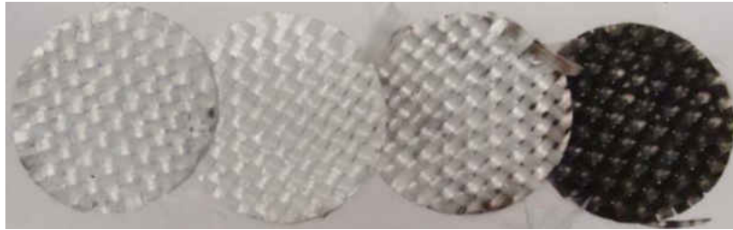
Figure 51 Residues of the composites after cone calorimeter tests.
