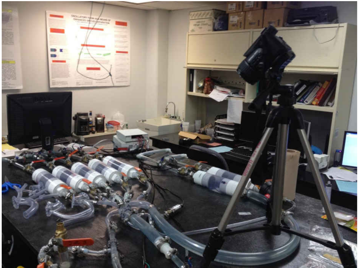
Figure 25: Camera apparatus for high FPS recordings of particles.
