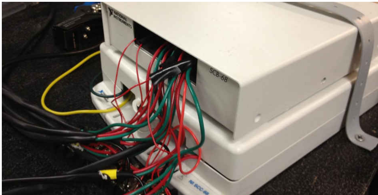
Figure 15: National Instruments terminal block.
