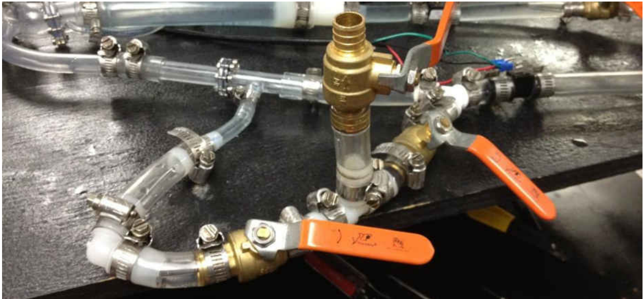
Figure 19: 3-valve injection system.
