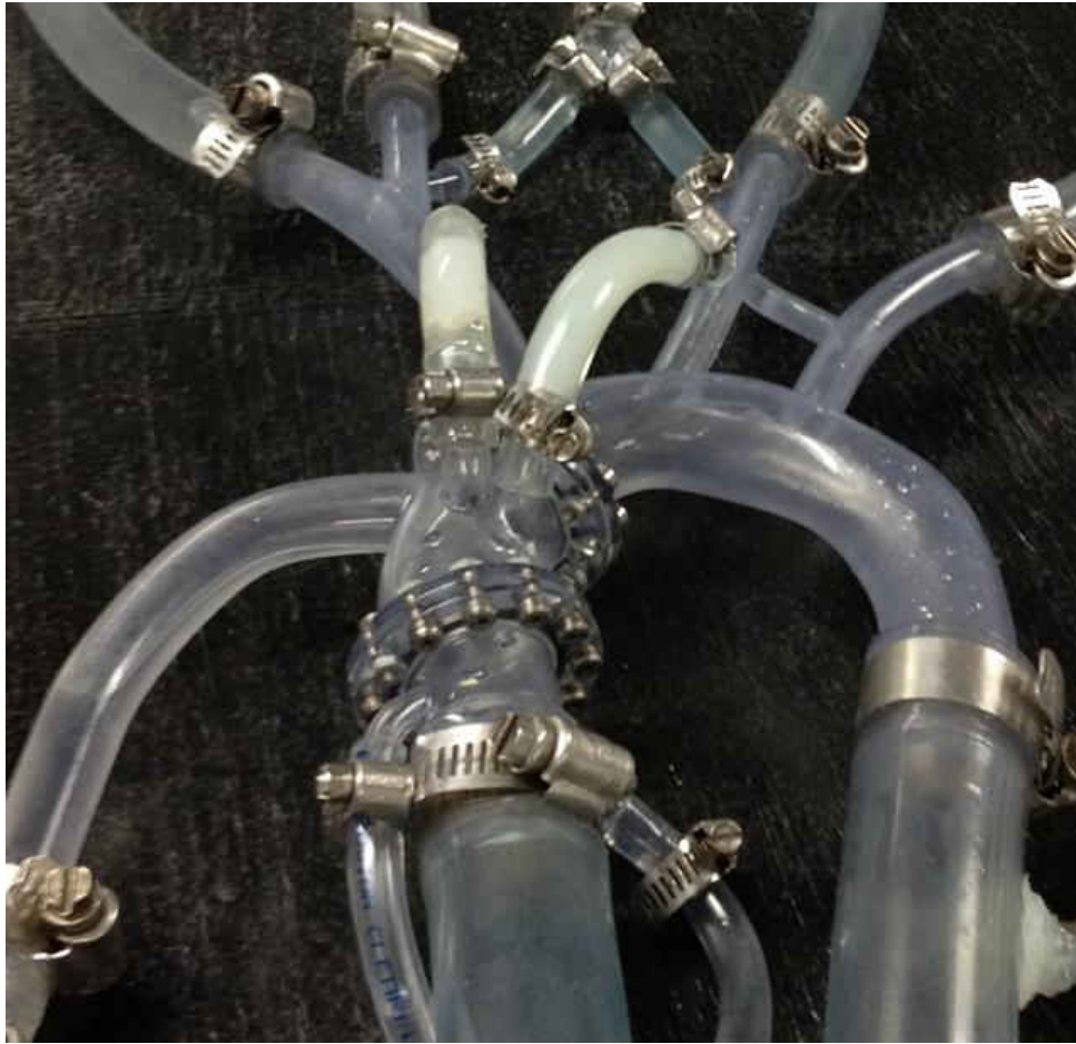
Figure 11: Printed rapid prototype part combined and attached to flow loop.
