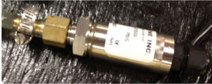
Figure 16: Pressure transducer attached near descending aorta.
