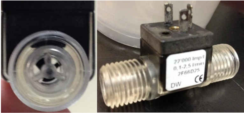
Figure 17: Cross section and side view of flow rate sensor.
