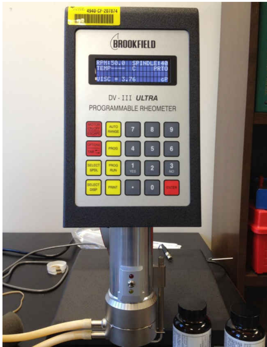
Figure 12: Viscometer with verified viscosity measurement.
