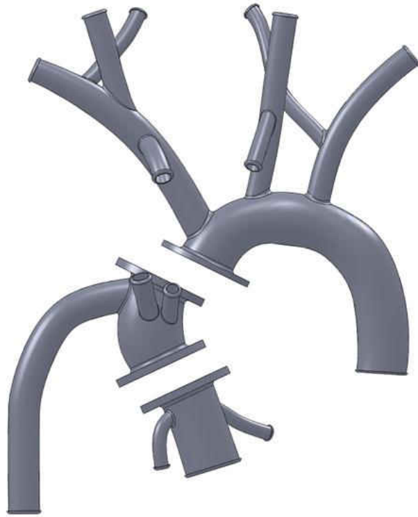
Figure 8: Converted CFD geometry to be rapid prototyped.
