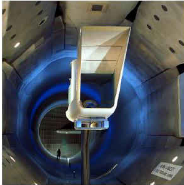
Figure 2.6: SAMPSON smart inlet testing in 16 feet transonic wind tunnel at NASA Langley [13].
