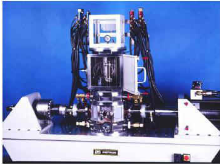
Figure 3.12: Load frame with high temperature furnace at SMARTS [43].
