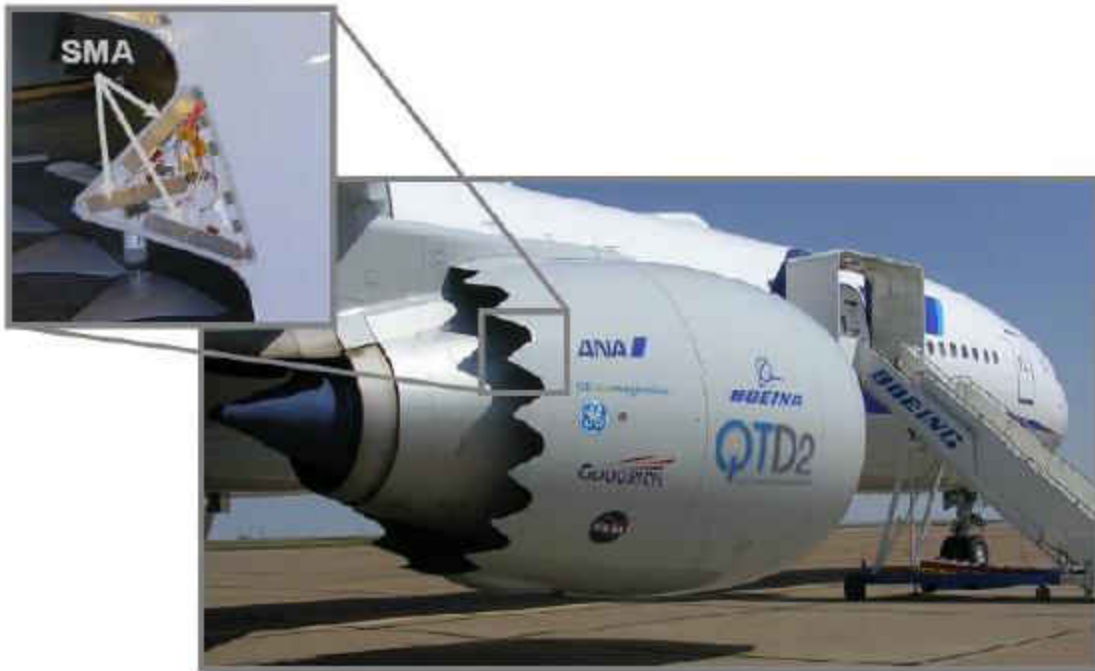
Figure 2.8: Variable Geometry Chevron (VGC) sleeve mounted on GE90-115B engine for 777-300ER flight test [1].
