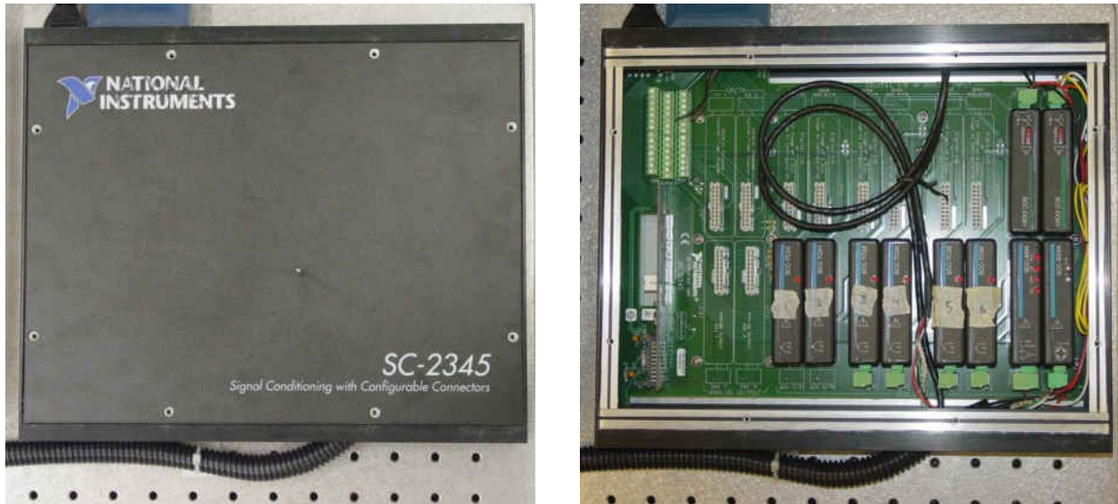
Figure 3.5: National Instruments signal conditioning carrier with various signal condition modules installed (see text for details).
