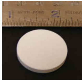
Figure 25: Optical photograph of as-coated EB-PVD TBC along with an inch scale.
