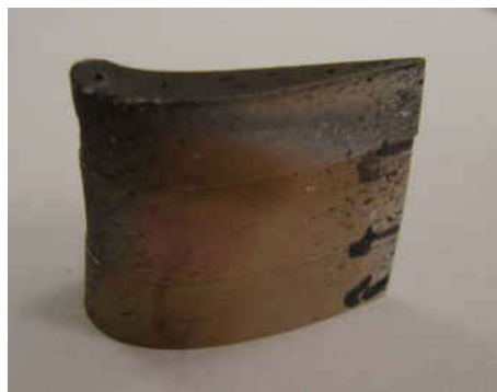
Figure 27: Optical photograph of serviced blade coated completely with colored deposit.
