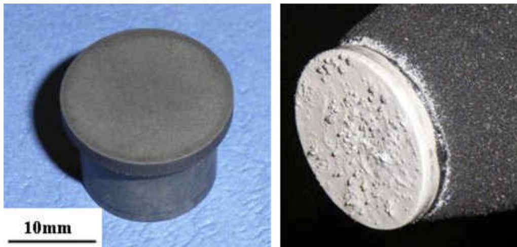
Figure 33: ZrB_2-20\%SiC specimen before (left) and after (right) oxyacetylene torch testing at 2200\text{ }^\circ\text{C} for 10 min [69].
