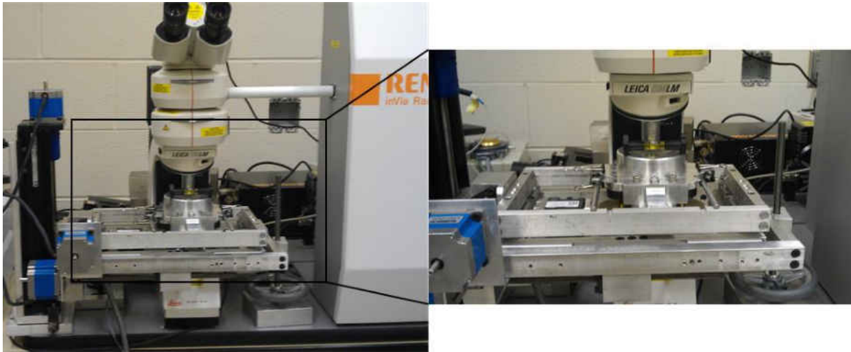
Figure 49: In-situ Raman Spectroscopy bending experiment Set-up
