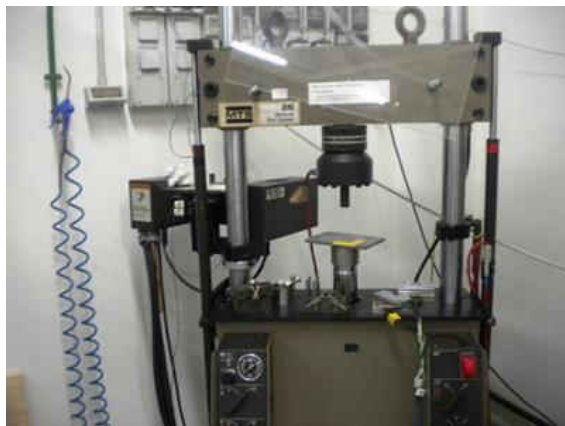
Figure 44: (a) MTS 810 system, (b) schematic diagram of the 4-point bending configuration, where H and B are the sample dimensions and L_1 is the loading distance and L_2 is the supporting span.
