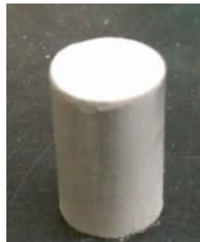
Figure 3.8: Ni-Ti sample after initial densification process
