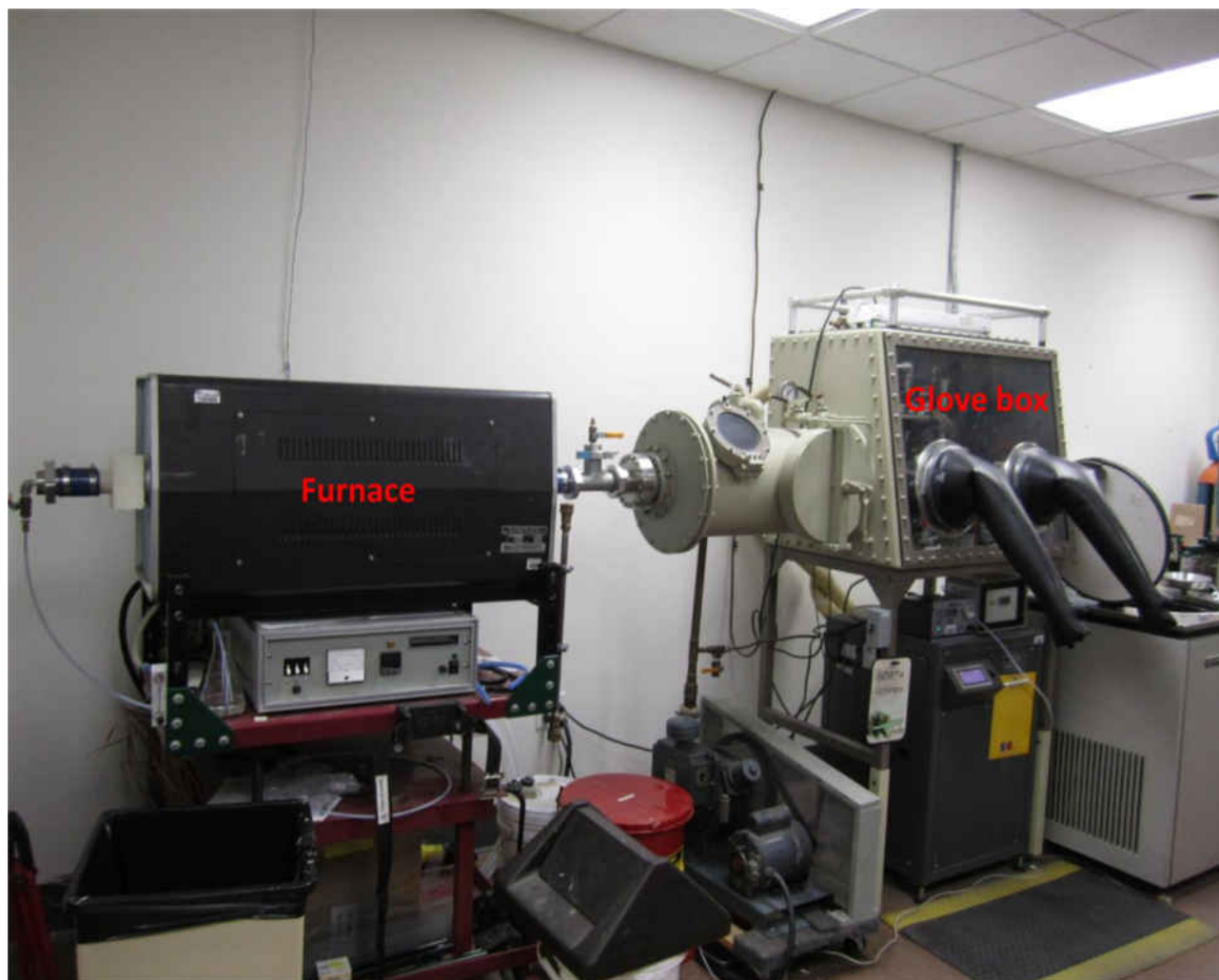
Figure 14: The glove box and furnace.
