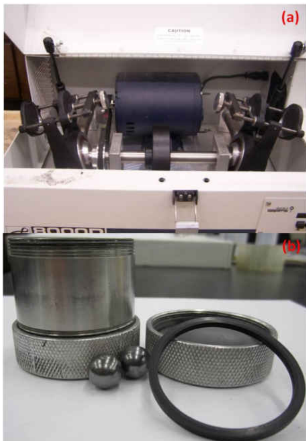
Figure 11: (a) Spex 8000 mixer mill and (b) milling vial and media.
