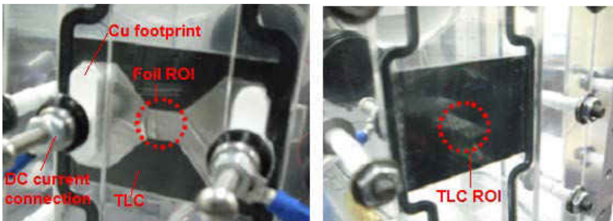
Figure 5: TLC and Fecralloy Heating Foil Combination; Boiling Activity ROI is shown
