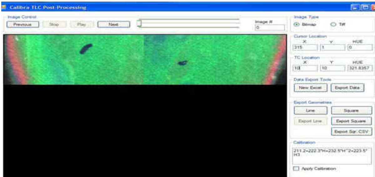
Figure 22: GUI Software Interface for TLC Image Post Processing
