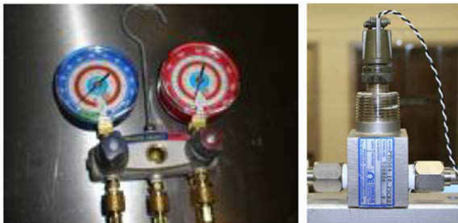
Figure 8: Experimental Equipment 3: Yellow Jacket Manifold (Left) and High Pressure Refrigerant Flow meter (Right)
