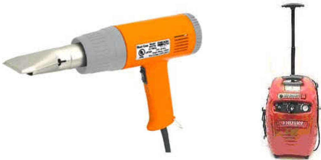
Figure 14: Experimental Equipment 9: Chicago Electric Power Tools Heat Gun #47269 (Left) and a Husky 1.5Gal 135psi Max Compressor (Right)
