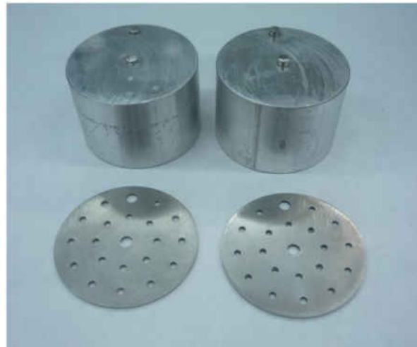
Figure 23. Specimen polishing jig
