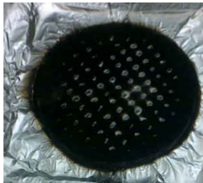
Figure 24: C25A sample after removed from the Cone Calorimeter experiment
